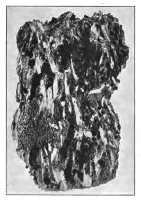
Fig. 41.—Portion of spruce pile destroyed in three years by marine borers in the harbor of Klawock, Alaska.
